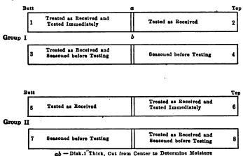
Fig. 16.—Method of cutting and marking test material.
